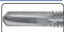
Sharp drill point & long flute length assures proper clearance of heavy gauge metal before any thread engagement begins.
