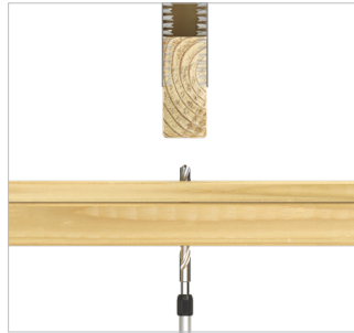
2 Predrill into top plate only
