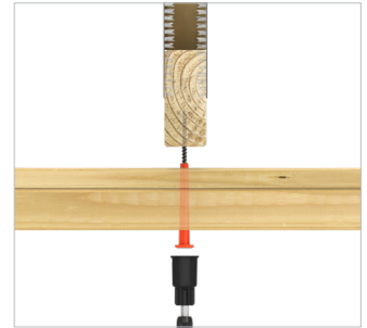
4 Drive SDPW Deflector screw through predrilled top plate and into the truss or ceiling joist
