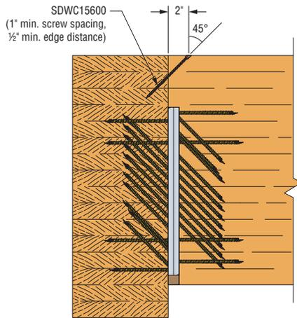
**ACBH3x15.37 Installation with SDWC15600 for Uplift Capacity (side view)**
