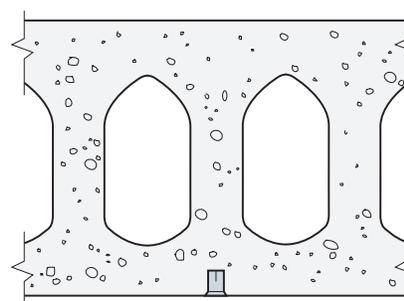
Figure 2. Hollow-Core Concrete Panel
