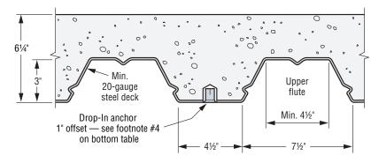
Figure 1. Lightweight Concrete over Steel Deck
