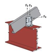
Typical FCB Installation for Roof Rafters
