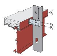
Typical FCB Installation at Bypass Framing
