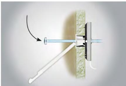
4. Snap off strap flush with collar. Insert the bolt through the fixture into the anchor and tighten securely.
