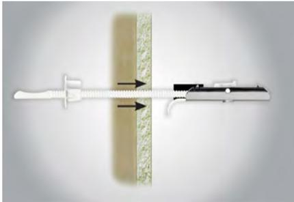
2. Insert the FlipToggle into the drilled hole. When the head is fully inserted, pull the strap to flip the toggle flat against the back of the wall.
