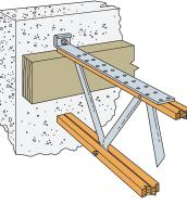
Typical LTTP2 Installation for I-joist
