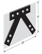
"W" and "H" indicate the envelope size of the steel shape.
