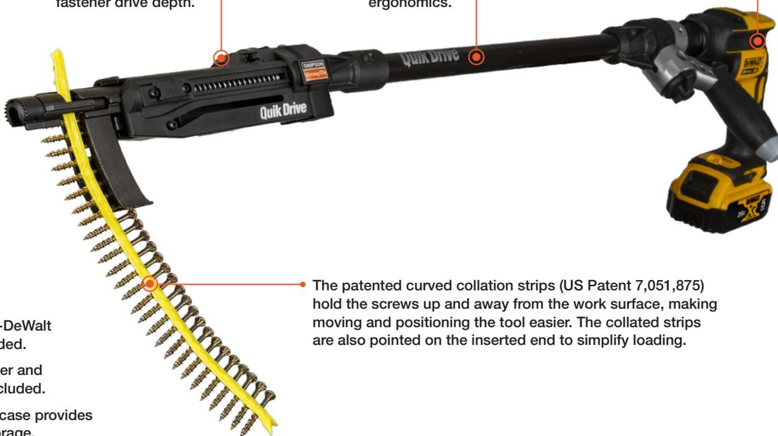
The patented curved collation strips (US Patent 7,051,875) hold the screws up and away from the work surface, making moving and positioning the tool easier. The collated strips are also pointed on the inserted end to simplify loading.
