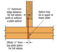
Min. Edge Distance for Top Plate Splice
