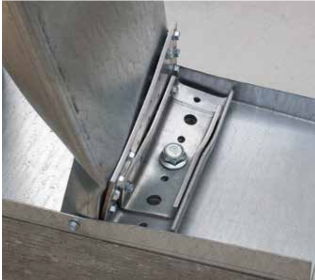
RCKW assembly test with member failure.
