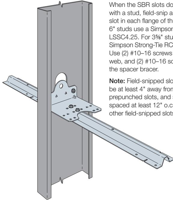
When the SBR slots do not line up with a stud, field-snip a ½"-deep slot in each flange of the SBR. For 6" studs use a Simpson Strong-Tie LSSC4.25. For 3½" studs use a Simpson Strong-Tie RCA223/54. Use (2) #10-16 screws to the stud web, and (2) #10-16 screws to the spacer bracer.
