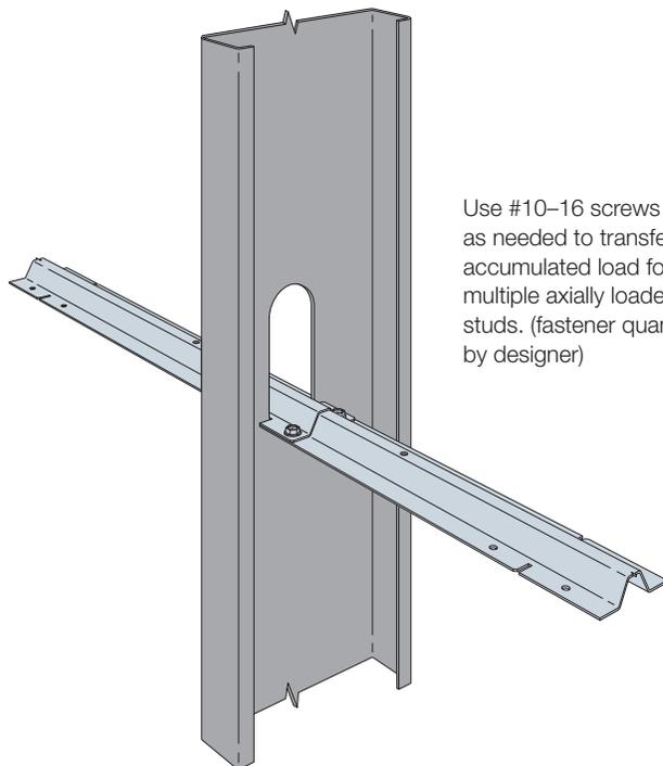
Use #10-16 screws as needed to transfer accumulated load for multiple axially loaded studs. (fastener quantity by designer)
