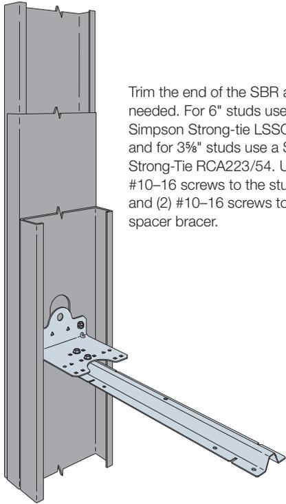
Trim the end of the SBR as needed. For 6" studs use a Simpson Strong-tie LSSC4.25 and for 3½" studs use a Simpson Strong-Tie RCA223/54. Use (2) #10-16 screws to the stud web, and (2) #10-16 screws to the spacer bracer.
