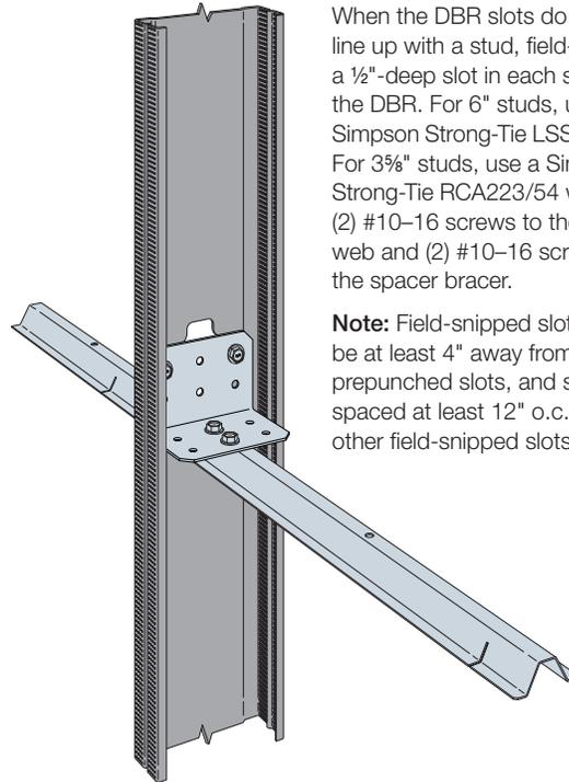
When the DBR slots do not line up with a stud, field-snip a ½"-deep slot in each side of the DBR. For 6" studs, use a Simpson Strong-Tie LSSC4.25. For 3½" studs, use a Simpson Strong-Tie RCA223/54 with (2) #10-16 screws to the stud web and (2) #10-16 screws to the spacer bracer.
