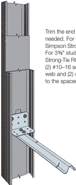
Trim the end of the DBR as needed. For 6" studs use a Simpson Strong-Tie LSSC4.25. For 3½" studs use a Simpson Strong-Tie RCA223/54. Use (2) #10-16 screws to the stud web and (2) #10-16 screws to the spacer bracer.
