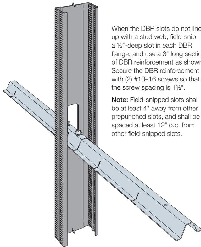
When the DBR slots do not line up with a stud web, field-snip a 1/2"-deep slot in each DBR flange, and use a 3" long section of DBR reinforcement as shown. Secure the DBR reinforcement with (2) #10-16 screws so that the screw spacing is 1 1/2".
