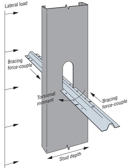
**Laterally Loaded C-Stud with SBR Spacer Bracer**
