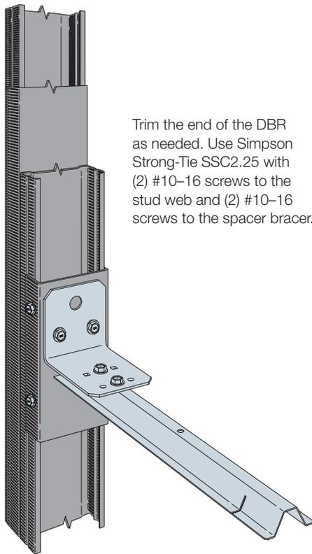
Trim the end of the DBR as needed. Use Simpson Strong-Tie SSC2.25 with (2) #10-16 screws to the stud web and (2) #10-16 screws to the spacer bracer.
