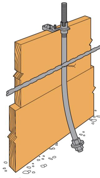
SB anchored using AnchorMate® at Embedment line (top of concrete)
