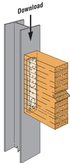
Beam to Steel Column Using SCBH3x15.37W-KT
