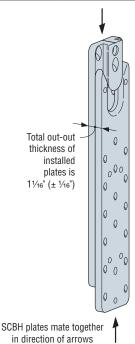
Assembly Thickness and Fit-up Tolerance
